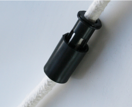
Close up of brake in it's engaged state
