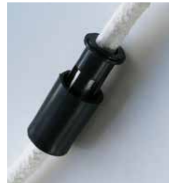
Close up of brake in it's engaged state
